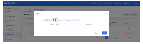
• If no upstream DHCPv6 server is available to assign the IP address, configure the IPv6 information as follows:
