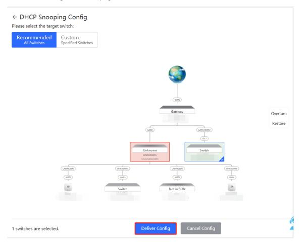
(3) After the configuration is delivered, if you need to modify the effective range of the anti-private connection function, click **Configure** to reselect the switch that enables the anti-private connection in the topology. After the configuration is delivered, if you want to modify the effective range of the DHCP Snooping function, click
